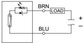
3. For solid-state type sensors, connect brown wire to the positive (+) and the blue to the negative (-) of DC power source. For 3-wire type, the black wire must be connected to the load only. If the black wire is accidentally connected to the power source, sensor may malfunction.
