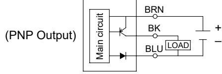
4. An external protection circuit may be required if the magnetic sensor is used with inductive load, such as relay or solenoid. For DC inductive load, attach an external diode parallel to the load and use R-C circuit parallel with AC inductive load as illustrated below.
