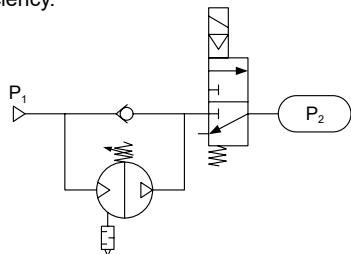
The inlet pressure ( $P_1$ ) first passes through a check valve to charge  $P_2$  until  $P_1=P_2$ .
